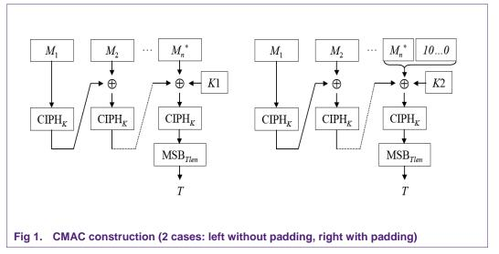
Fig 1 illustrates the standard CMAC constructions (see [CMAC]) in two possible padding cases.
